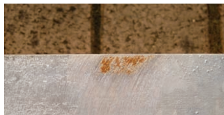
Zinc rich paint used on damaged galvanized coating – before and after
