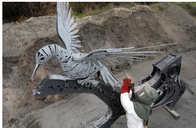
Removing the flaking paint by sand blasting
