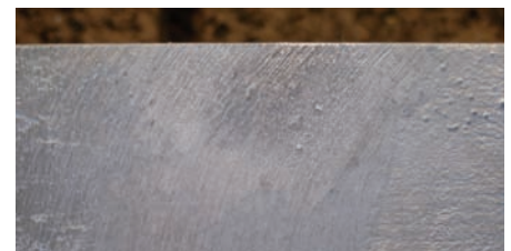
Zinc rich paint used on damaged galvanized coating – before and after
